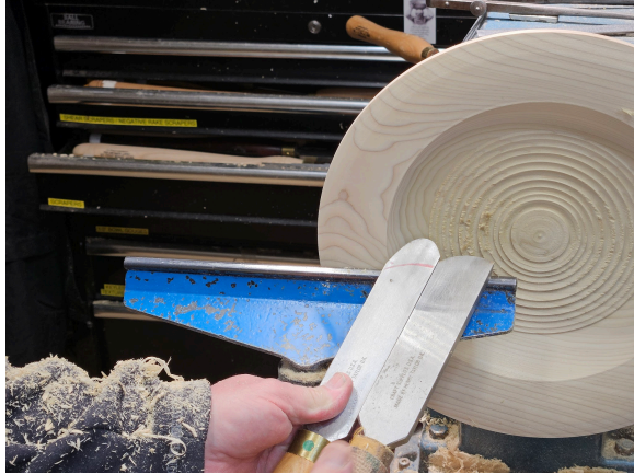
Fig 45 When using any scraper, lift the tool rest so that the tool handle is pointing down hill. The higher the handle is raised the less aggressive the tool becomes. (Fig 45)
