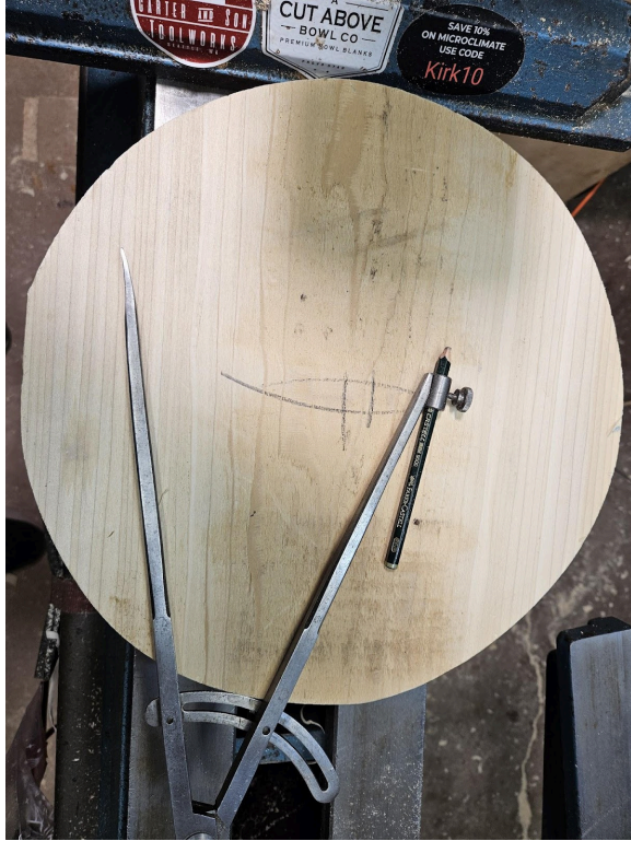
Fig 11 This will give us a rough center. We can now drill a hole at the center of the small square. (Fig 12)
