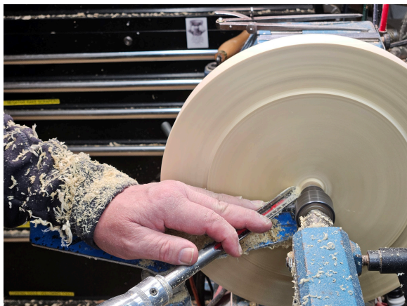
Fig 25 The foot ring should be slightly cut deeper toward the center. (Fig 26)
