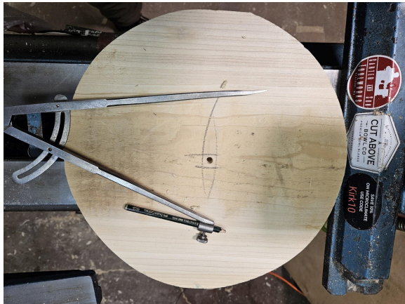
Fig 11 This will give us a rough center. We can now drill a hole at the center of the small square. (Fig 12)
