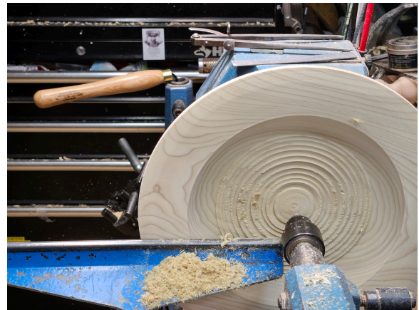
Fig 44 This is a spot where a heavy scraper could be used to refine the curve in the bowl of the platter. Choosing the right scraper, the French curve scraper shown on the left has a much tighter curve than the Radius scraper on the right. It is better to use a scraper that has a radius similar to the curve in the bowl. If we choose to use the French curve, we are most likely to leave more ridges than the larger Radius scraper (Fig 45)
