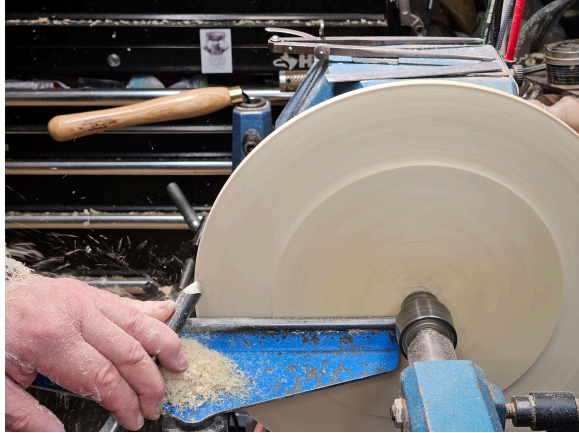
Fig 41 Forming the other side of the bead by turning the tool over for a bevel riding push cut towards the center, and starting at the top of the bead 1/3rd in. The rim on this platter will be about 1/3rd of the radius.(Fig 42)
