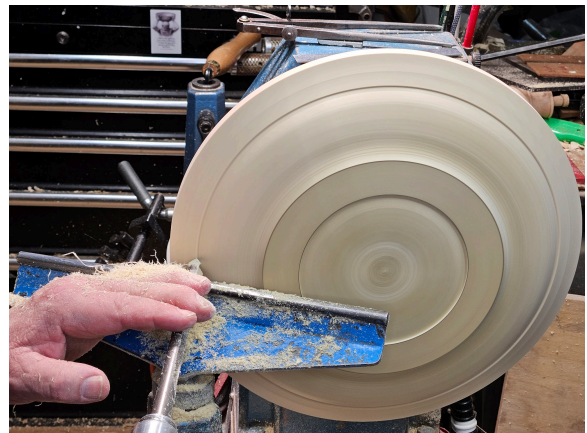
Fig 33 As the cut gets deeper at the bottom of the cove, the cut is stopped, the gouge turns over and cuts a straight line or fillet to separate the ogee. (Fig 34)
