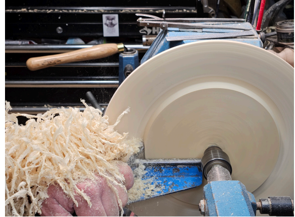
Fig 43 This is a very efficient way to remove the wood from the bowl of a platter, because the platter is flatgrain. This is not the way to hollow a deeper bowl. With a deeper bowl there is a much higher risk of hitting endgrain. (Fig 44)
