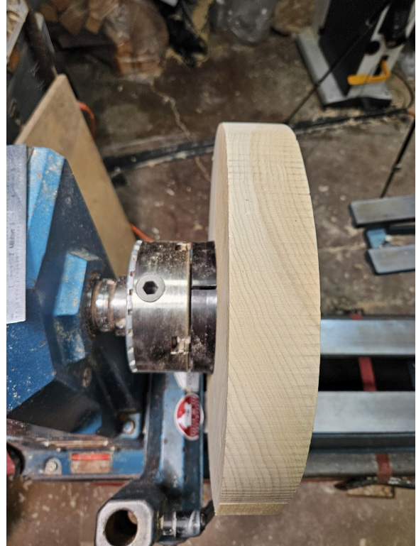
Fig 13 Make sure that the blank is tight to the chuck jaws. As noted before I am using a larger set of jaws this will add much needed stability to dampen vibration as we cut the back of the platter.
