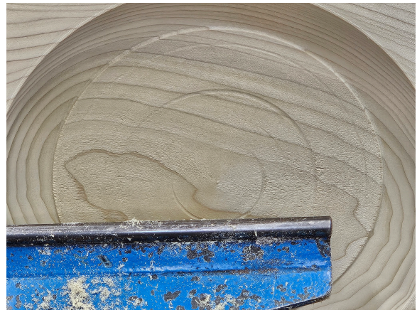
Fig 47 And then follow up with a gouge for a clean cut. Since this is all flat grain, a traditional ground bowl gouge AKA "Bottom feeder" is the preferred choice. (Fig 48)
