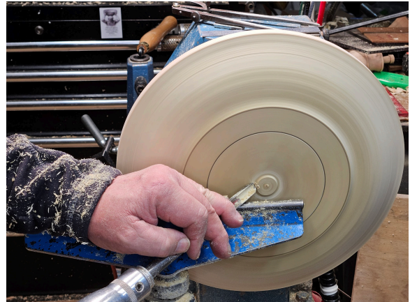
Fig 32 Cutting from the center to the chuck spigot straight across. This will form a spigot 1/8" deep. This is enough for my chuck jaws to grab and I want to be close to the closed diameter of the jaws. This will give me the best bite from the jaws. I use a small scraper to finish the spigot. A skew or gouge could also be used. Next cut is a bevel riding cut just under the surface of the ogee curve. From the foot ring to the rim. (Fig 33)
