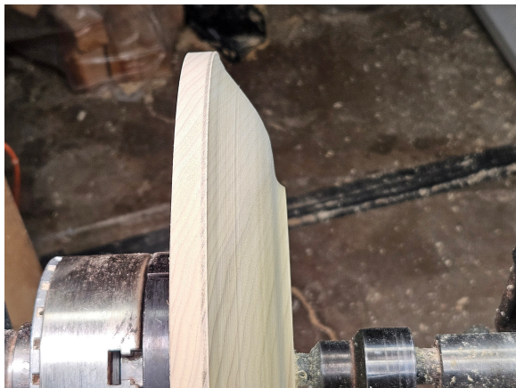
Fig 31 Cut in the spigot by cutting slightly deeper as you go toward the center. Note: I don't cut deeper than 1/8" (Fig 32)
