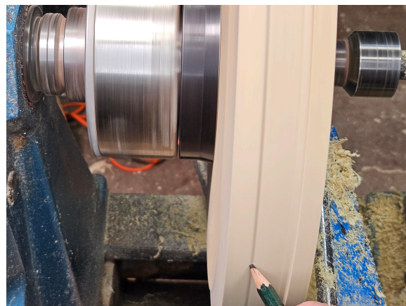
Fig 28 Cut a cove from between the lines. (Fig 29)
