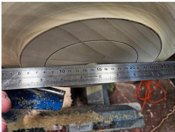
Fig 26 Split the remaining wood from the foot ring to the rim in 3rds in (Fig 27) I am using a golden mean caliper to find 1/3rd from the
