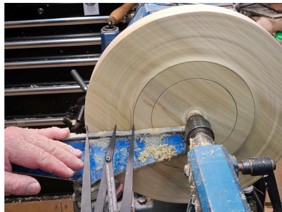
Fig 27 Mark a line \frac{1}{2} inch from the top down on the rim. Note: don't push the pencil in hard, you might need to sand this line out. (Fig 28)
