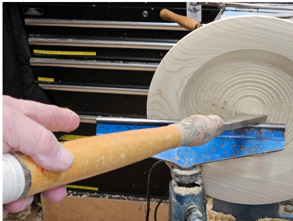
Fig 45 One of the tradeoffs that we have to consider when using a scraper is that they might lift grain. In this piece of softer density wood (Tulip Poplar) It is very common to have the grain lift (Fig 46) many turners like to use Negative rake scrapers. Not shown. Because they are less aggressive than traditional scrapers. It was not considered for this piece. Because of the soft density of the wood. Negative rake scrapers work best in hard density woods.
