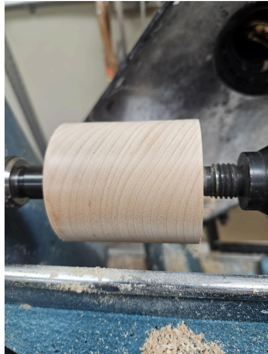
Fig 2 Round over the lead edge. We want to have a soft round corner. (Fig 3)
