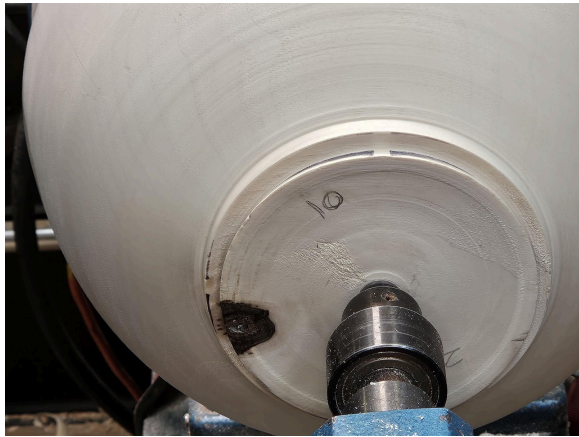
Fig 52 Use the tailstock as an insurance policy as long as you can. Removing it to have full access to the bottom of the bowl. (Fig 53)
