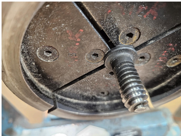
Fig 5 With the screw installed in the chuck set a pair of dividers to the size of the jaws that are suited for the blank that you are using. A good rule of thumb is to have 40% of the diameter in the chuck. (Fig 6)
