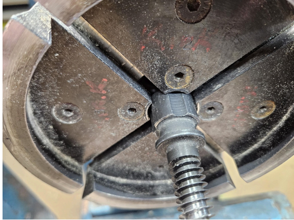
Fig 4 Next we want the jaws to be in the groove in the screw. (Fig 5)
