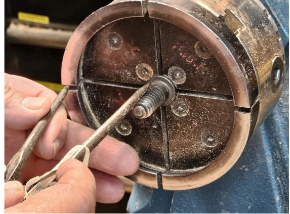
Fig 6 It's time to drill the appropriate drill hole. I use a hand drill with a collar on the bit. I don't want the hole deeper than needed for the screw because I core most of my bowl blanks. (Fig 7)
