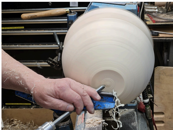
Fig 52 Use the tailstock as an insurance policy as long as you can. Removing it to have full access to the bottom of the bowl. (Fig 53)
