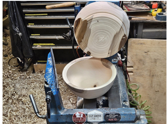
Fig 55 Using the jamb chuck Start your next project or reuse the jamb chuck on other bowls.
