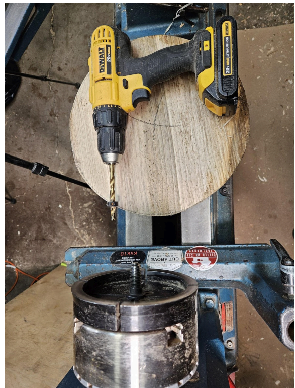
Fig 7 Mount the blank onto the screw. I do this with the lathe running at a speed less than 350 rpm . It's a bit like feeding a horse. Keep your hands open, don't grip
