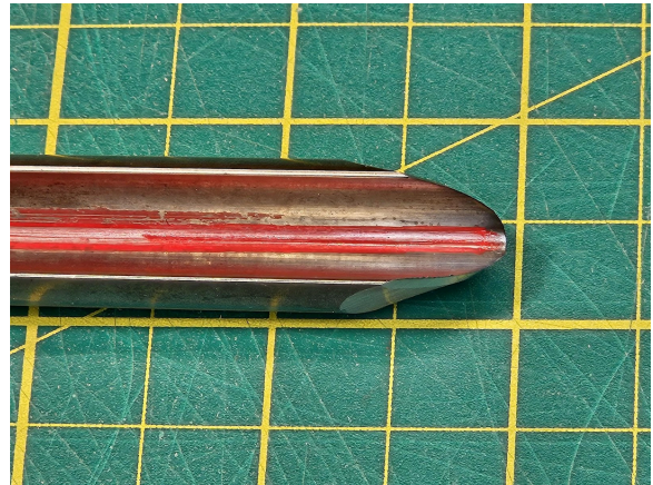
Fig 10 The micro bevel helps in several ways(Fig 11) First the sharper secondary bevel is sharpened first with a coarse grinding wheel in order to remove material fast! And leave less material to grind with the finer wheel extending the life of the finer wheel. And perhaps the most important reason is that it doesn't leave as deep of compression marks on the inside of a bowl. When sharpening any tool, keep your hands away from the wheel. (Fig 12) I choke up on the tool and jig, keeping my hands free of the wheel if the tool should slide off the wheel. I like to keep my elbows close to my side.
