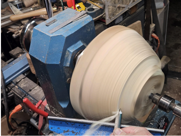
Fig 18 This is the shaving that should be coming off your tool.
