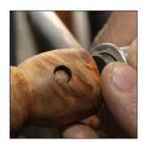
6. Finish shaping outside of acorn body and sand. Clean dust from inside, wax threads and interior, then part off.
