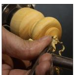
12. Stipple cap surface using chatter tool or texturing tool. Shape top of cap, leaving top stem 3/16" thick, and part off.
