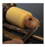
11. Shape cap to match body, then remove body. Cut away extra threads leaving two near cap, finish cut the cap base, wax the threads.
