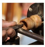
5. Hollow remainder of body with round-nose scraper. Refine inside of bird entrance hole with round grinding bur in Dremel, then carefully sand interior, not touching the threads.
