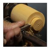
9. Slow lathe speed to 300-450 rpm. Top of male thread chaser must be on center line or slightly below. Start with tool handle angled toward tailstock and chamfer angle. Begin moving tool lightly to the left, cutting half thread each pass, bringing the cutting edge parallel to the wood as you work along the tenon. Pull the tool off the thread
