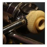
13. Make threaded jam chuck from scrap wood (or your next acorn body) and screw in cap. Finish cut the cap top, leaving stem 1/8" diameter.
