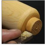
10. Test fit acorn body and recut threads until body screws on loosely, fitting flush to cap. Screw body on cap, finish cut the point, and sand. Apply finish to acorn body now, if you like.
