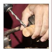
2. True up the top of the acorn body, then bore a 3/8" hole to the inside bottom depth. Hollow 2/3 deep inside with round-nose scraper, leaving rim 1/8" thick and parallel side 1/4" deep.
