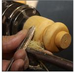
8. Angle tenon edge slightly and cut groove using 3-point tool in corner where tenon meets cap.
