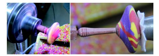
Wet sand the clay disk with wet or dry sandpaper, or micro-mesh cloth. I dip the sandpaper into water and then apply it to the disk. Using Micro-mesh, you can sand to 1500. Depending on how well you conditioned the clay, and removed air bubbles, the surface of the clay will be smooth with a semi-gloss finish.
