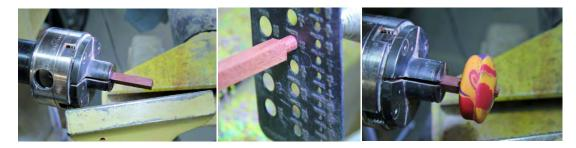
Turn the bottom inch of the stem round where the clay disk will be glued. Using a drill guide as a gauge, I can be sure I will have a nice tight fit when I drill a hole through the clay disk.
