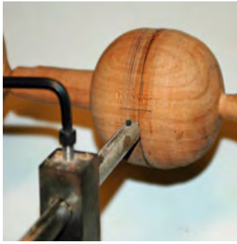
Photo 20 Center cutter to the glue line of the sphere
