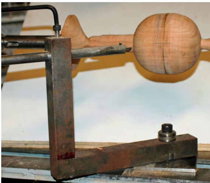
Photo 18 Home made sphere cutter
