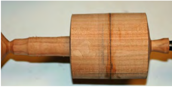
Photo 15 Rough the stem down to size
