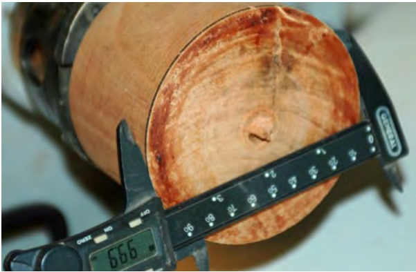
Photo 7 Measure outside diameter, inside 6mm less
