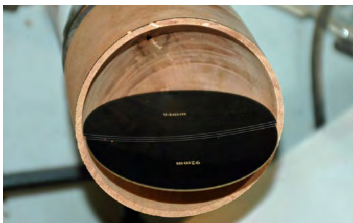
Photo 10 Cut the inside to the first line on guide
