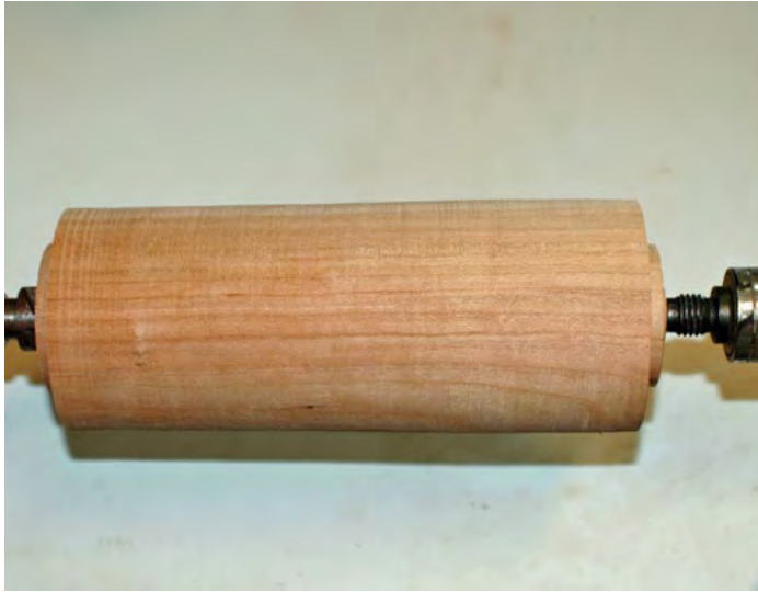
Photo 4 Rough your wood to a cylinder
