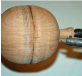
Photo 21 Slide cutter outward until it clears all wood
