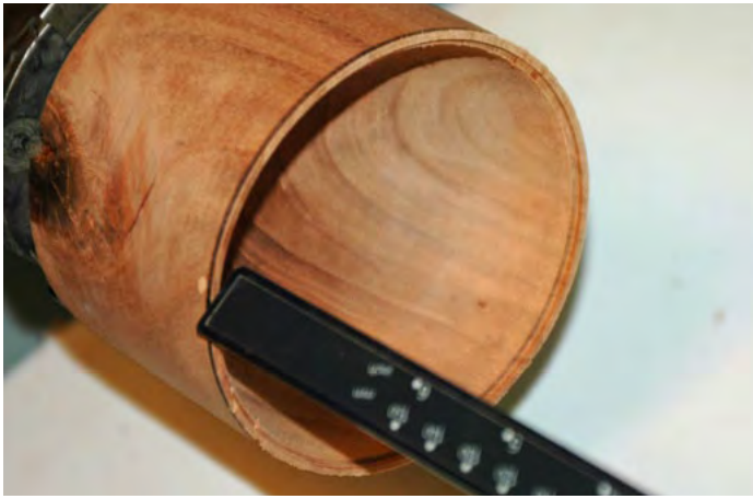
Photo 11 Cut a 2mm step on the inside of the top
