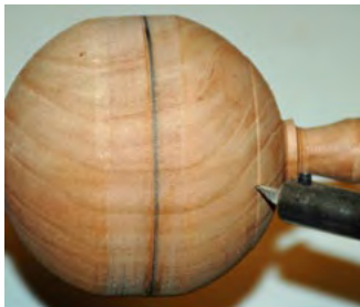
Photo 22 Adjust cutter to take a small bite per pass
