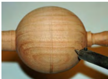
Photo 23 Continue until the glue line cleans up
