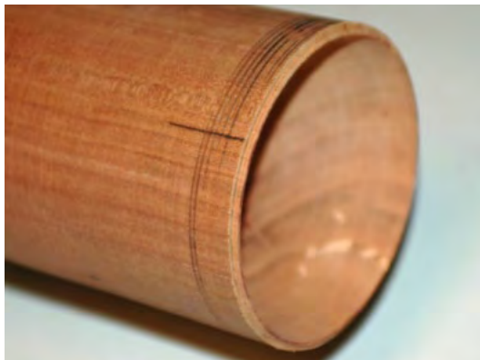
Photo 13 Cut a 2mm stem on the outside of bottom
