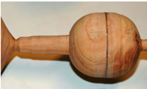
Photo 17 Rough the corners with a gouge
