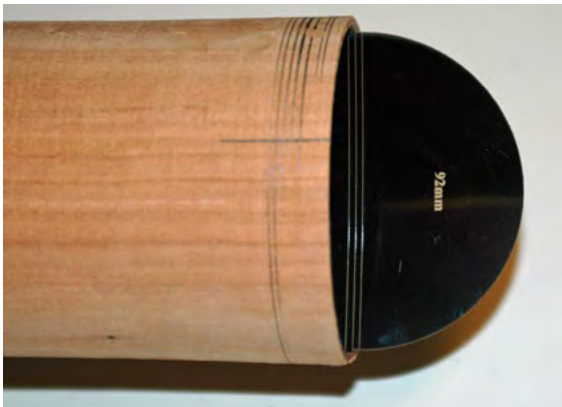
Photo 12 Cut bottom 2mm deeper than the top
